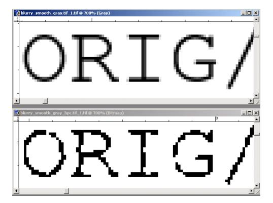
In the images above, we see that when the Bits per Color Channel argument is set equal to 1 (-bpc=1) we lose all the gray values from the smoothing operation. The glyphs end up looking grainy and spotty as a result.
